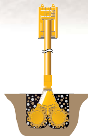
CSM Cutter-Soil-Mixing
