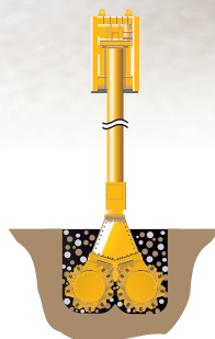
CSM Cutter Soil Mixing
